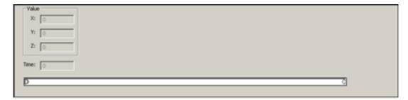
• Emitter\_Rate: Allows you to adjust the Emitter rate. Possible values are anywhere from 0 to 10000. In essence, this setting determines how many particles are emitted per second. The following is a screen-shot of the Keyframe Editing Window when the Emitter\_Rate property is selected. Left-click in the graph to insert new keyframes. Right-click on keyframe handles to remove them.
